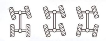
Equipped with three steering modes: four-wheel steering, crab steering, and front-wheel steering, the boom lifts are also capable of one-touch wheel alignment.
